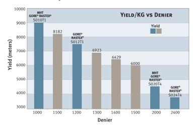
Because of its high yield, lower denier MHT GORE® RASTEX® Sewing Thread can provide lower cost per meter than many higher denier threads.
