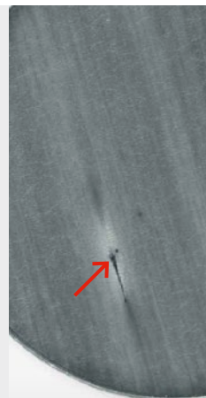
Figure 1: Not acceptable — pin hole in vent
