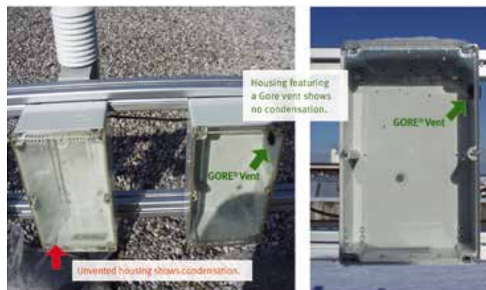
Figure: Long-term study of pressure differentials in electronics housings
