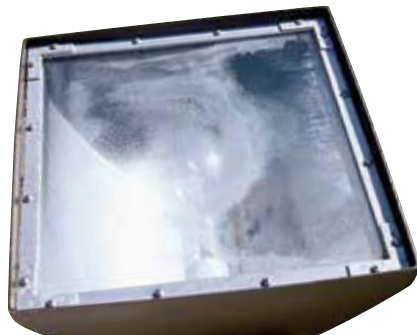
Figure: Luminaire with condensation
