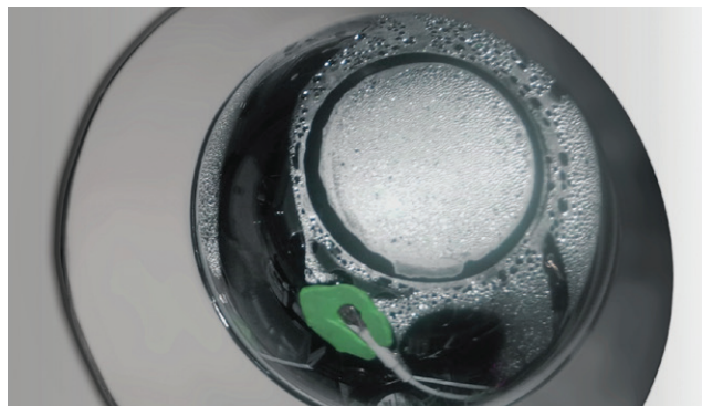
Figure 1: Desiccant could not prevent severe condensation from forming and becoming trapped within this sealed enclosure.
