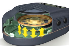
Transducer bias created by pressure on compliant surfaces
