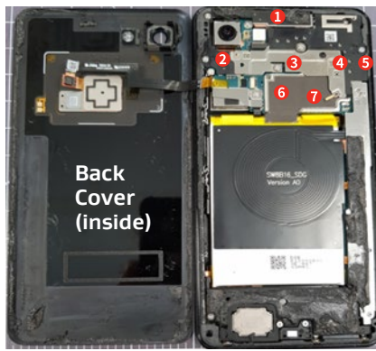
Figure 9: Google Pixel 3XL with back cover removed. Existing air gap thickness measured by conformable polymer at seven locations shown.
