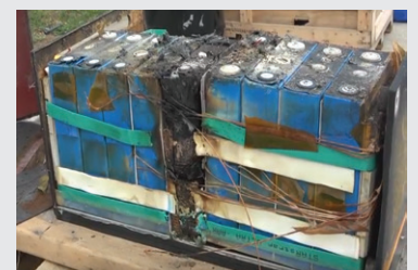
Figure 5: BESS Module (Our Next Energy, Inc.) Post-Thermal Runaway Test using GORE Battery Insulation
