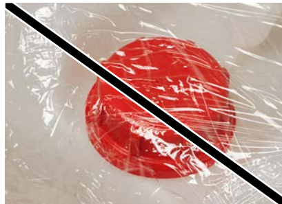
Venting holes blocked by foil
