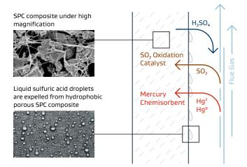
The SPC composite captures and sequesters elemental and oxidized mercury while converting  $SO_2$  to liquid sulfuric acid.
