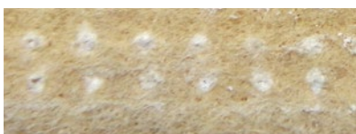
TiO 2 particulate migration through unsealed stitch holes within 4 months of service.
