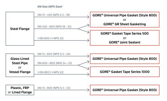
These selection criteria are for general guidance only. To determine suitability in a specific application, see the product data sheets and installation instructions on gore.com. If additional assistance is needed, please contact GORE® Gaskets Technical Support.
