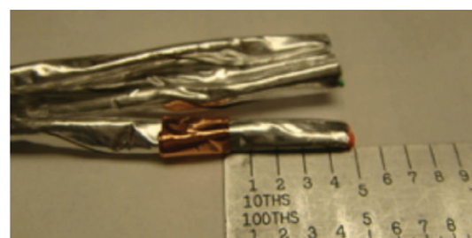
Figure 16: Wrapping the foil
