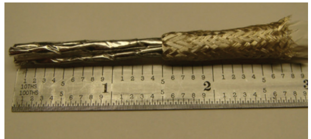
Figure 15: Exposing the foil
