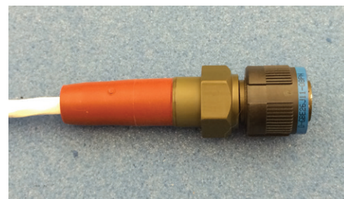
Figure 27: Affixing the backshell
