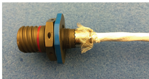
Figure 42: Trimming the excess braid material
