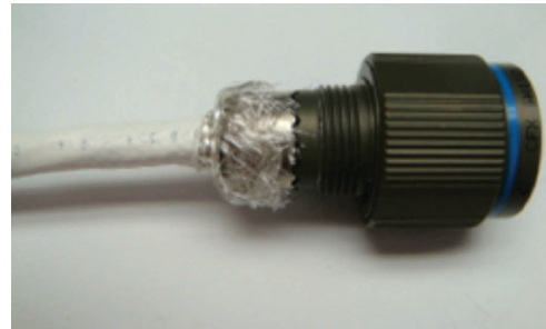
Figure 25: Trimming the excess braid material
