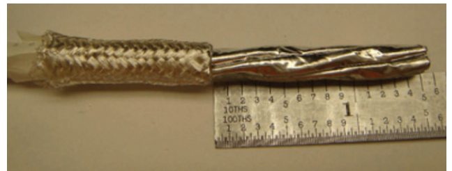
Figure 32: Exposing the foil
