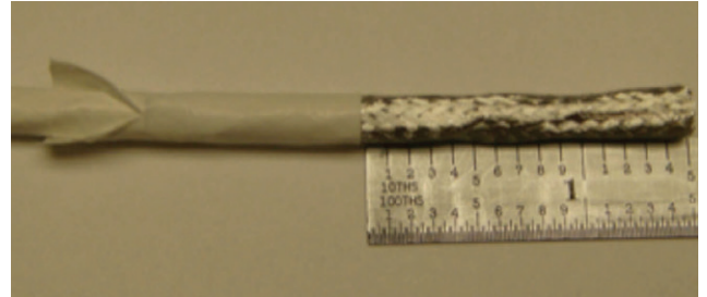
Figure 31: Exposing the braid
