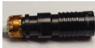
Figure 49: Taping microband on plug
