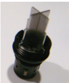
Figure 37: Replacing the crossbar
