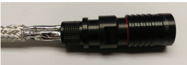
Figure 25: Seating the backshell
