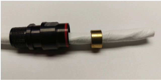
Figure 11: Sliding components onto the cable
