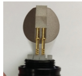
Figure 39: Using contact insertion tool
