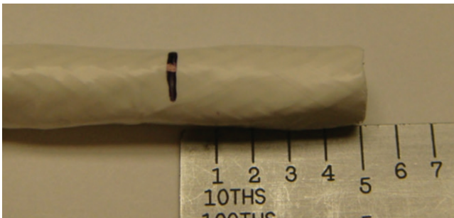
Figure 12: Marking the cable
