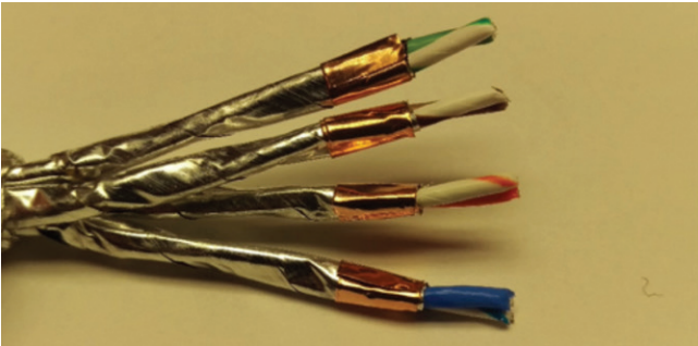
Figure 17: Removing the foil edge
