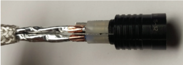
Figure 23: Inserting the back insulator
