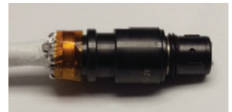
Figure 50: Taping microband on socket
