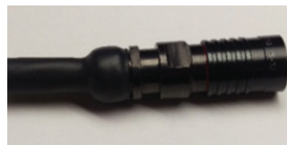
Figure 51: Shrinking tubing on plug backshell
