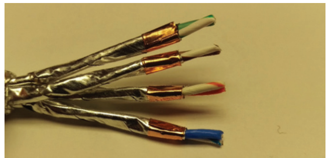
Figure 34: Removing the foil edge
