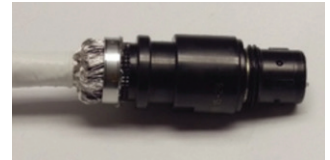
Figure 48: Trimming excess braid on socket
