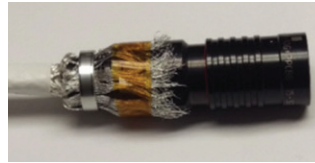
Figure 45: Attaching microband to plug
