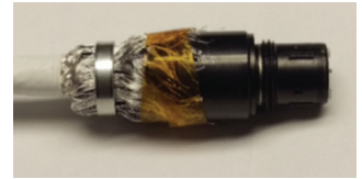
Figure 46: Attaching microband to socket
