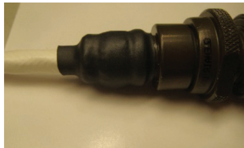
Figure 73: Shrinking tubing over backshell
