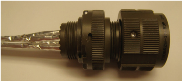
Figure 37: Connecting the grommet to the plug
