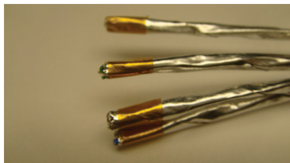
Figure 47: Taping each pair
