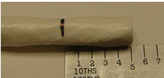
Figure 11: Marking the cable
