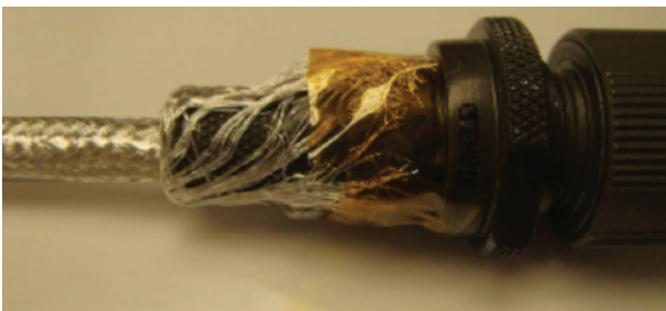
Figure 38: Returning braid to connector
