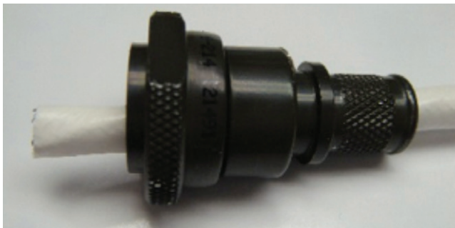
Figure 42: Inserting backshell on the cable
