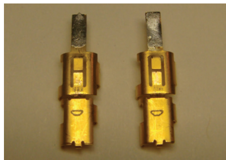
Figure 27: Tinning ears of outer body
