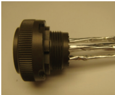
Figure 17: Pairs inserted in connector grommet
