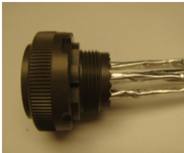
Figure 49: Pairs inserted in connector grommet
