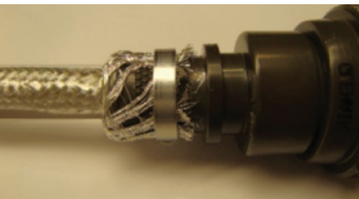
Figure 71: Attached Band-It® clamp
