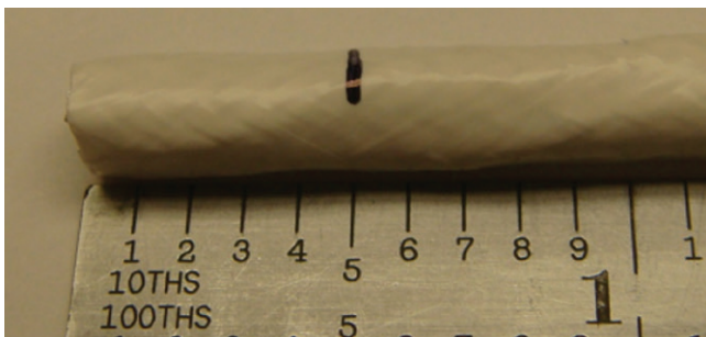
Figure 43: Marking the cable
