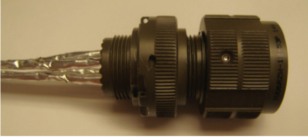
Figure 69: Connecting the grommet to the receptacle
