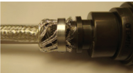
Figure 39: Attached Band-It® clamp
