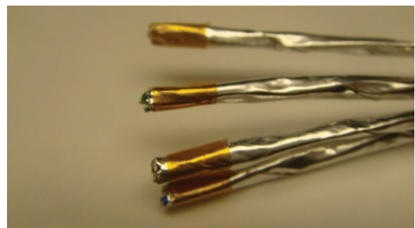
Figure 15: Taping each pair
