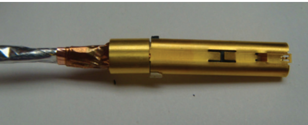
Figure 64: Positioning the ferrule
