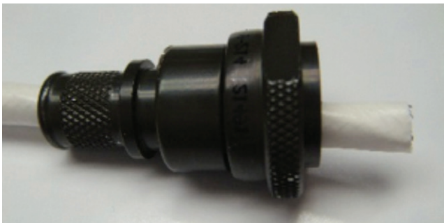
Figure 10: Inserting backshell on the cable
