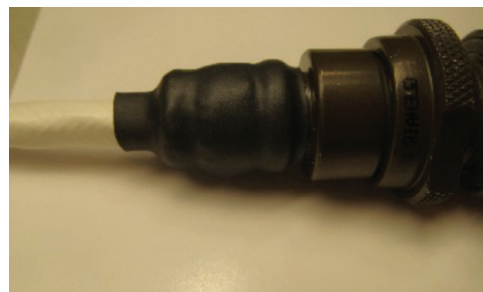
Figure 41: Shrinking tubing to backshell
