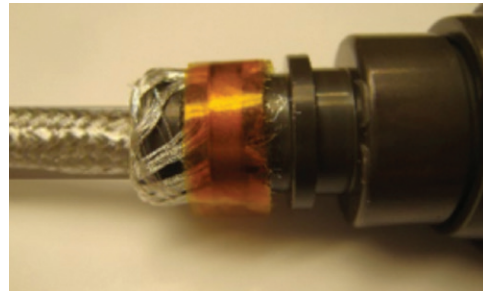
Figure 40: Wrapping Band-It® clamp
