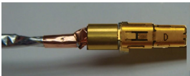
Figure 32: Positioning the ferrule
