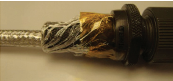
Figure 70: Returning braid to connector
