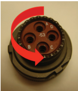
Figure 16: Inserting each pair into connector grommet
