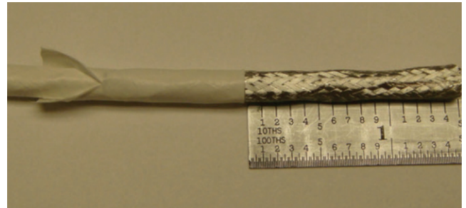
Figure 11: Exposing the braid
