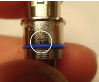
Figure 35: Engraved pin number
