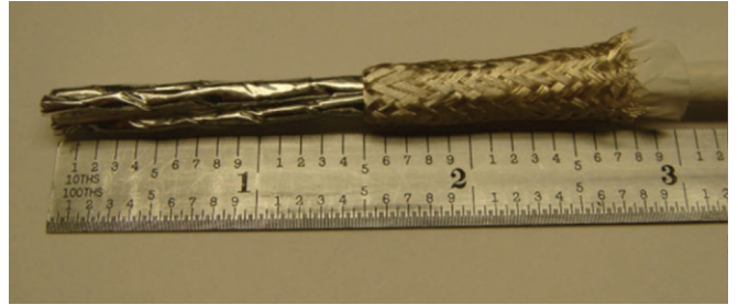
Figure 29: Exposing the foil
