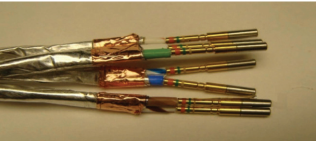
Figure 33: Stripping the contacts
