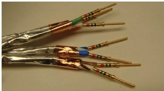
Figure 16: Stripping the contacts
