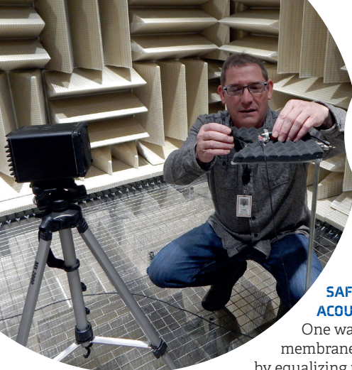
Left: Acoustic testing inside Gore's anechoic chamber
