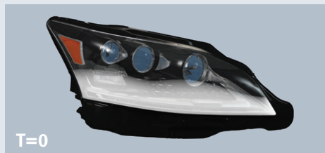
Lamp B – Final clearing time: 20 minutes
