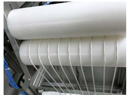
No Jacket Breakage (BS/SWS) during TicToc-Test > 1 MM Cycles
