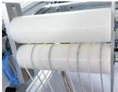
Jacket Breakage Breakage (VEN2) during TicToc-Test < 1 MM Cycles
