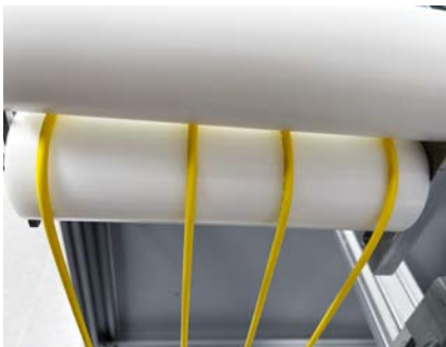
No Jacket Breakage (VEN1) during TicToc-Test > 1 MM Cycles
