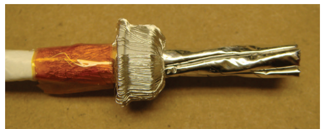
Figure 18: Securing the braid wire ends
