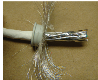
Figure 17: Sliding the support sleeve
