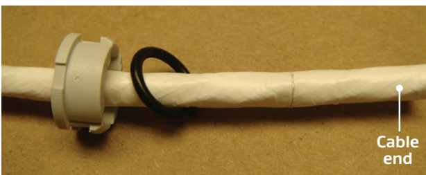
Figure 48: Sliding the O-ring
