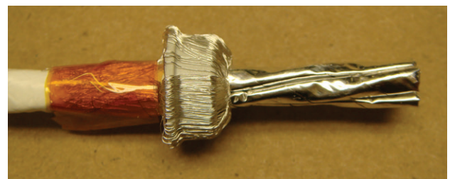
Figure 57: Securing the braid wire ends
