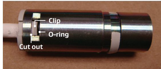
Figure 43: Lining up the clips with cutouts
