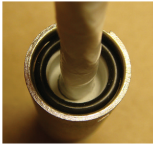
Figure 42: O-ring fully seated
