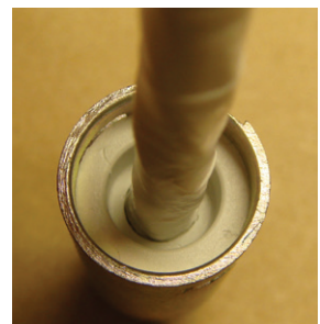
Figure 80: Support sleeve in connector body
