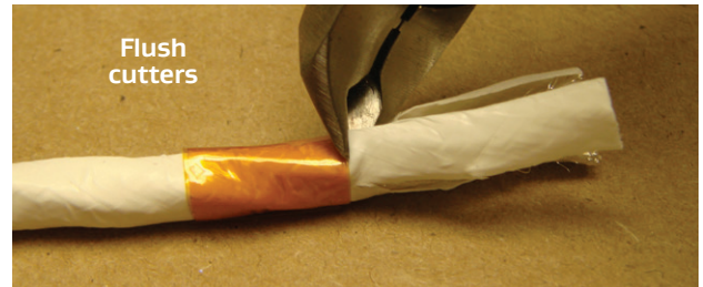
Figure 55: Cutting the two flaps
