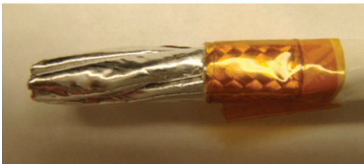
Figure 7: Removing the braid
