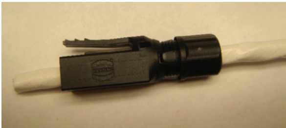
Figure 5: Attaching the labels, sleeving and black housing
