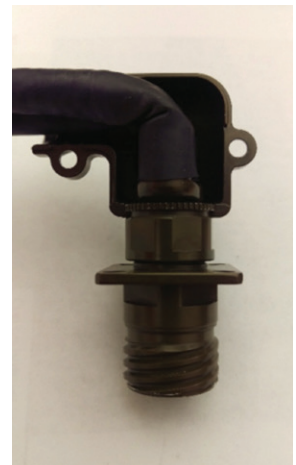
Figure 52: Attaching right-angle backshell
