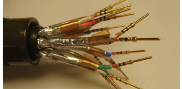
Figure 24: Stripping the primaries
