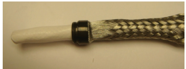
Figure 30: Inserting cable into braided shield
