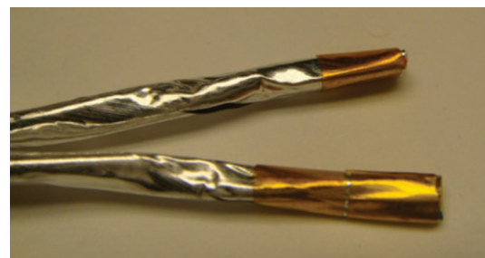
Figure 20: Wrapping the foil
