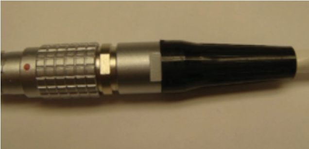
Figure 44: Installing the connector cap on plug end
