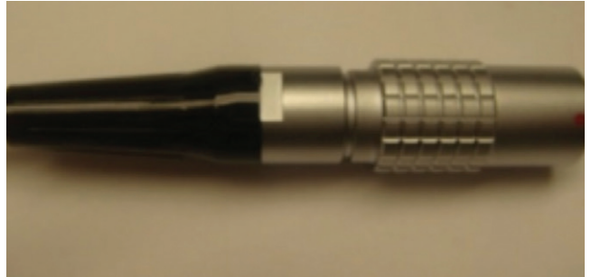
Figure 45: Installing the connector cap on socket end
