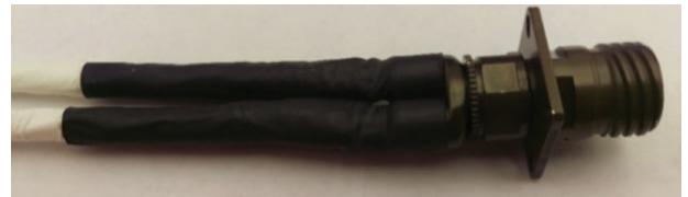
Figure 50: Covering the receptacle with TAT material
