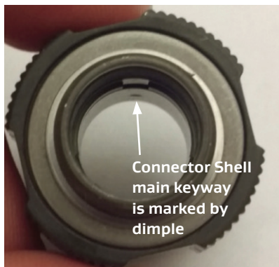
Figure 29: Inserting connector shell on cable
