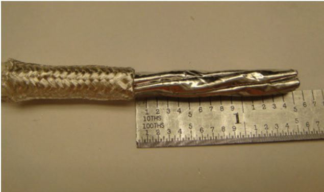
Figure 10: Exposing the foil
