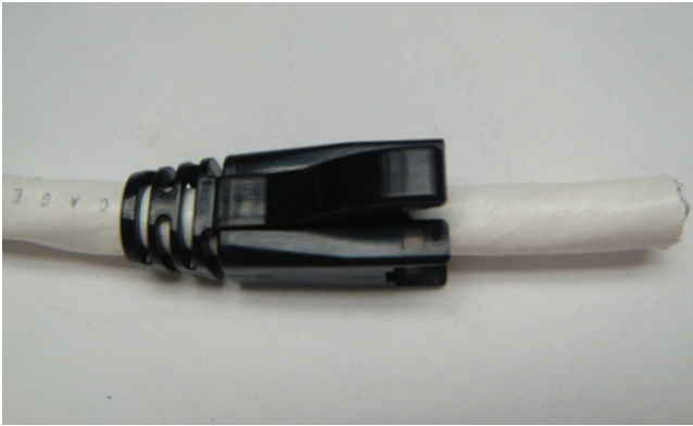
Figure 6: Attaching the strain relief grommet
