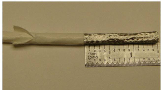
Figure 9: Exposing the braid
