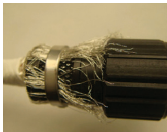
Figure 43: Attaching Band-It to plug
