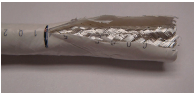
Figure 12: Slitting the cable jacket
