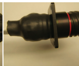
Figure 50: Shrinking tubing on receptacle
