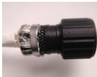
Figure 45: Trimming excess braid on plug
