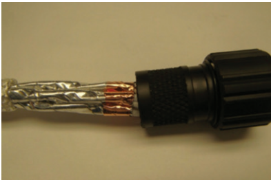
Figure 24: Inserting primaries into the connector
