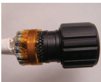
Figure 47: Taping the plug
