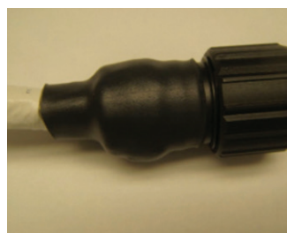
Figure 49: Shrinking tubing on plug
