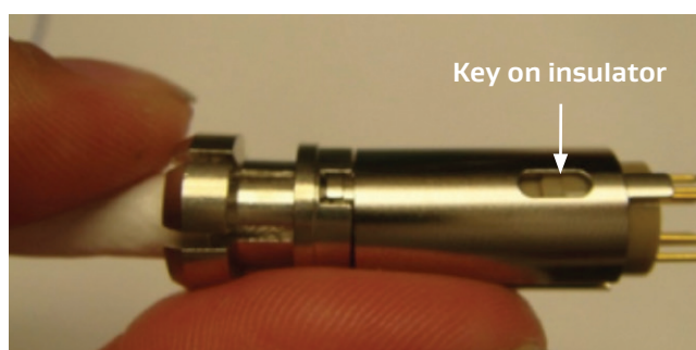
Figure 43: Insulator key for alignment
