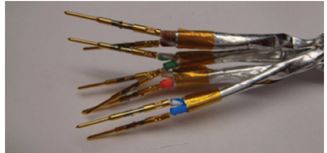
Figure 17: Stripping the pairs
