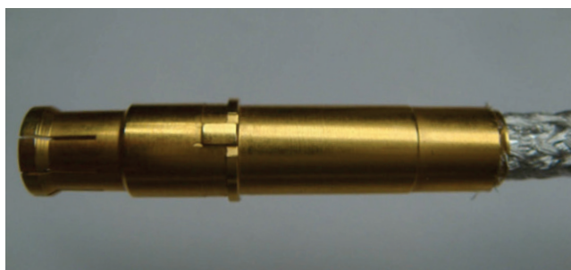
Figure 57: Trimming the braid
