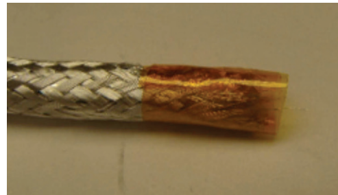
Figure 14: Taping the braid end
