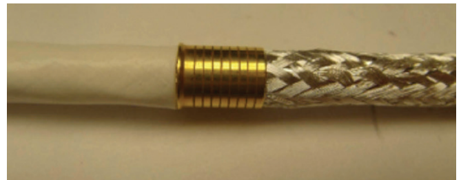
Figure 15: Sliding crimp ferrule on cable
