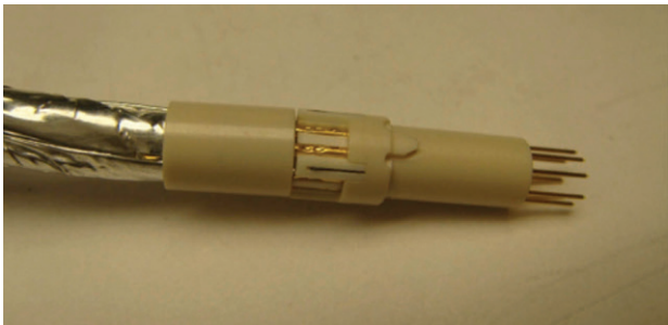
Figure 26: Returning the plastic bushing
