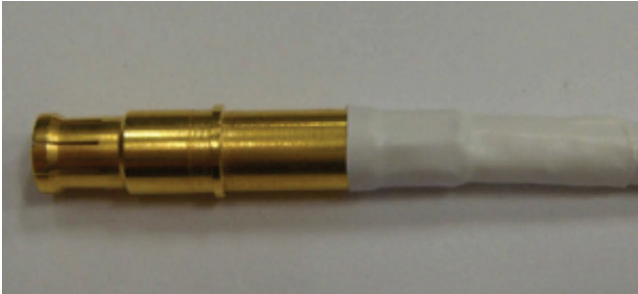
Figure 62: Shrinking tubing on crimp socket
