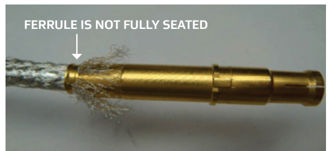
Figure 32: Pushing the ferrule
