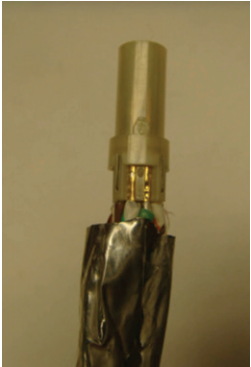
Figure 49: Seating the outer insulator
