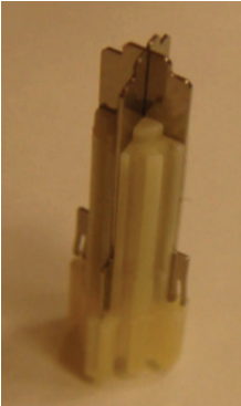
Figure 22: Inner insulator with metal spacers
