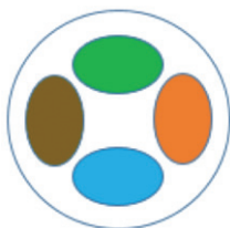
Figure 9: Pairs configuration at plug end
