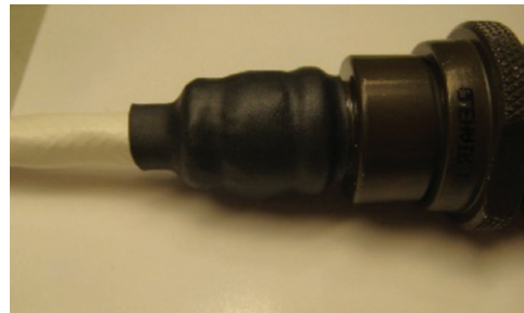
Figure 73: Shrinking tubing over backshell
