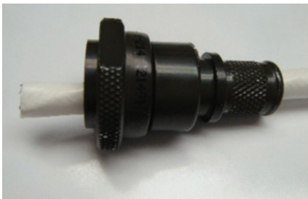
Figure 42: Inserting backshell on the cable
