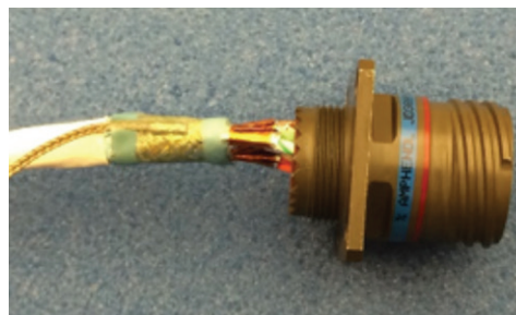
Figure 45: Returning the outer jacket
