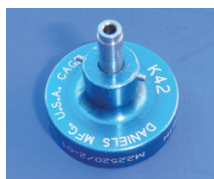
Figure 5: Pin positioner (K42)
