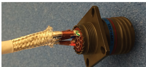
Figure 41: Trimming the braid
