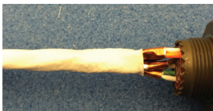
Figure 27: Returning the outer jacket
