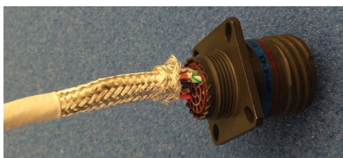
Figure 40: Sliding the braid back
