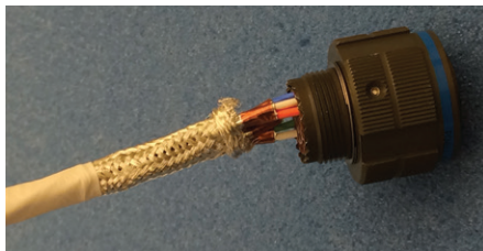
Figure 24: Sliding the braid back
