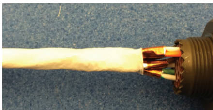
Figure 43: Returning the outer jacket
