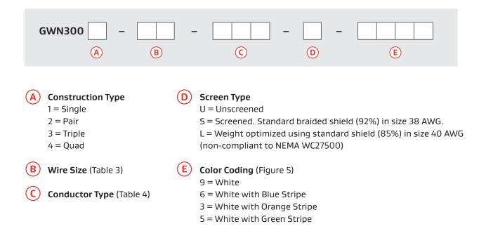
Gore's part number GWN3002-20-NCC-S-96 is an example that meets MIL-STD-104 Class 2 requirements. It includes a standard shielded twisted pair in size 20 AWG with solid white and white with blue stripe color coding and ETP copper nickel-plated conductors. Per NEMA WC 27500, only combinations 9, 96, 963, and 9635 are possible (Figure 5).
