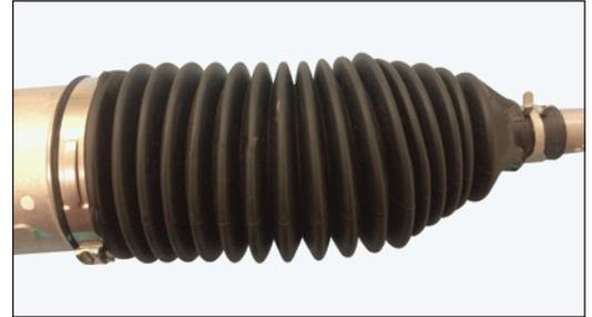
Venting prevents deformation, preserving the boot’s structural integrity and reliably maintaining its “as-designed” protective function.
