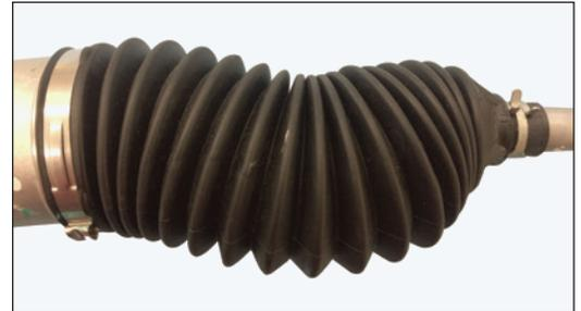
Sealed systems “trap” pressure differentials that cause boot deformation.
