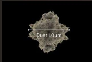
IP6x admits small (1-10 µm) particles like dust.
