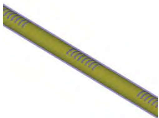
Figure 6 A length of leaky feeder with alternating leaky and shielded sections.
