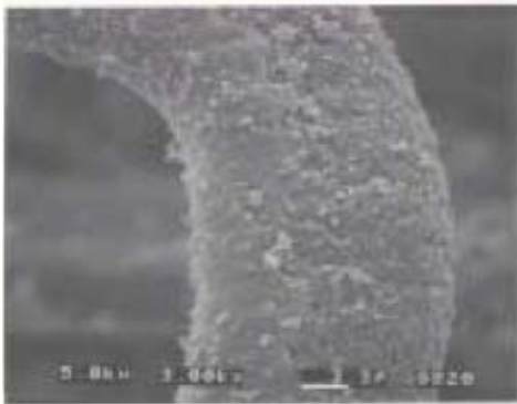
Figure 2: Surface morphology of used fiber at 3,000x magnification
