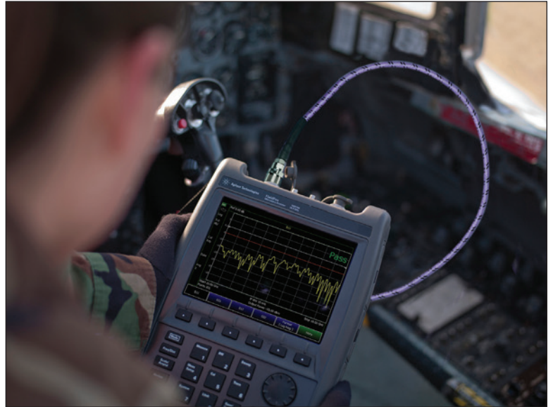
Figure 2. FieldFox Handheld RF and Microwave Analyzer used during Flight Line Testing. (Image Courtesy of Keysight Technologies)
