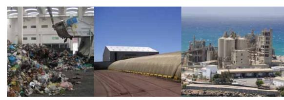
processed through the GORE® Cover system with a short exposure time to achieve <20% moisture content and a calorific value of >20Mj/kg. The result will be grinded to pieces smaller than 30 mm and the outcome is directly sold to feed energy intensive industries, like the cement industry.
