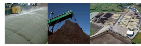
technology. As a result there are more than 150 plants worldwide with throughputs of 6,500 t/a up to 600,000 t/a operating with our technology, and licensed to operate in accordance with Odour and Emission Control Laws. The combination of a membrane cover and controlled aeration allows a reliable composting process. Pressurised aeration ensures a sufficient supply of oxygen and
