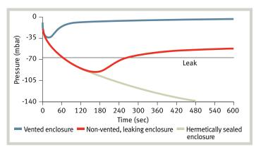
In non-vented housings, 70 mbar (1 psi) of pressure causes seals to leak after repeated temperature cycles. Vented housings equalize pressure and prevent seals from leaking.
