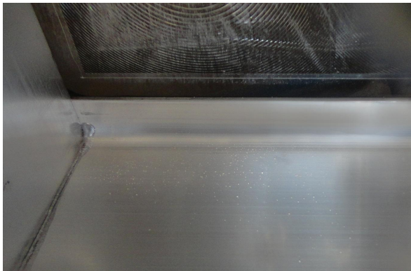
FIGURE 7. Dust Collected on Lens.
