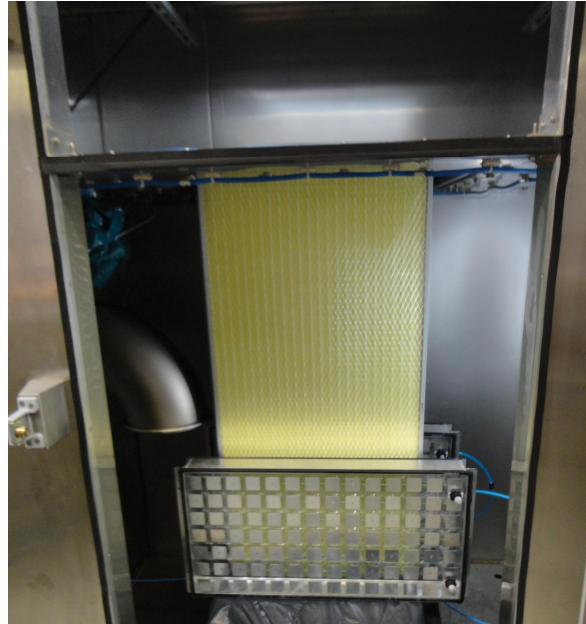
FIGURE 3. Test Chamber With Two of Soitec's Concentrix™ CX-M400 Modules.
