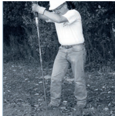
1 A 1,5 cm diameter hole is placed 60–100 cm into the surface.
