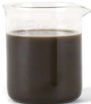
Actual compressor cleaning fluid after just 1450 hours use of conventional F9 filters.
