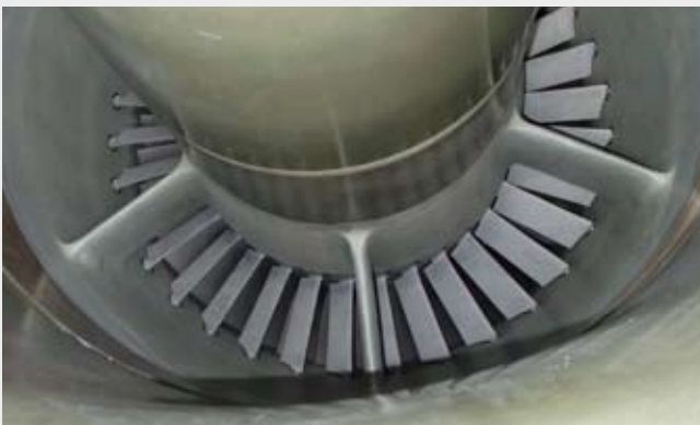
Clean intake after 7600 hours runtime with GORE® Turbine Filters without off-line washings.
