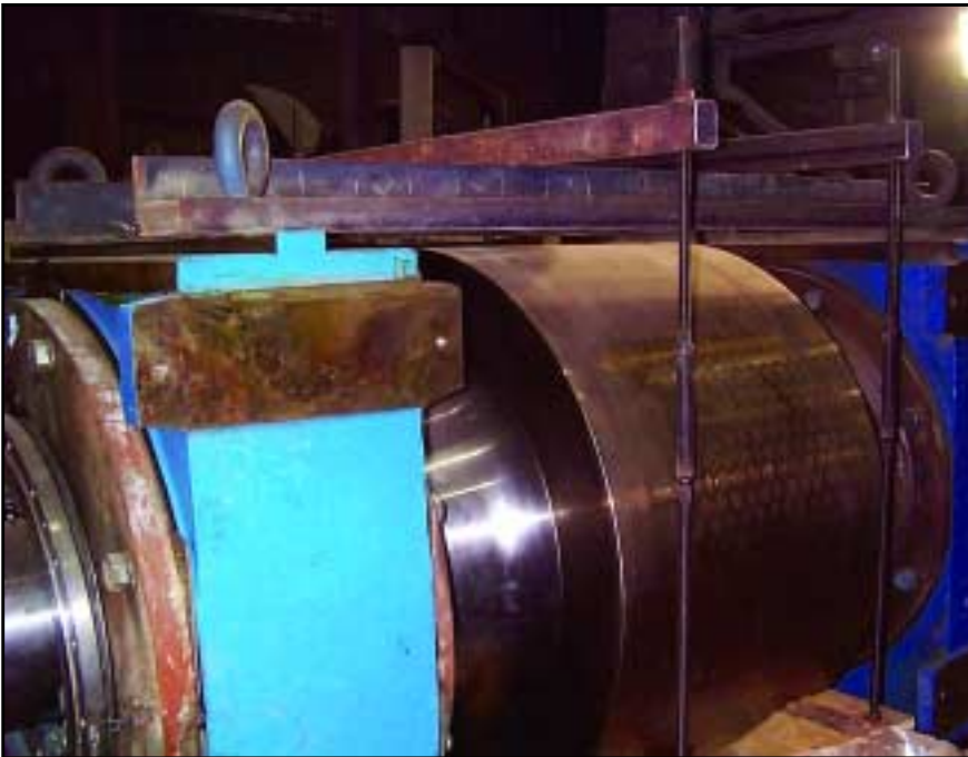
Masch. Koppern's Hexadur tyres and rollers for the hydraulic roller press.
