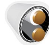
Part Number: 108 Shielded Signal Cable 2x AWG 24 shielded twisted pair Ratings: 450V rms Dimensions: 2.2 mm +/- 0.0 mm (0.087 in +/- 0.000 in)
