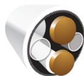
Part Number: 107 Shielded Signal Cable 2x AWG 20 shielded Ratings: 600V rms Dimensions: 3.3 mm +/- 0.1 mm (0.130 in +/- 0.004 in)
