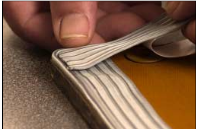
SKYFLEX ® aircraft sealant is being installed around the corner of the panel. Notice that the sealant has been overlapped. By using the proper installation technique, water ingress will be prevented from reaching the structure.
